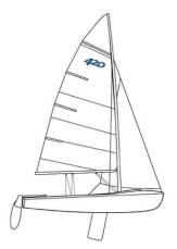
The **Club 420** Class Dinghy is a double-handed (2 crew) monohulled planing dinghy with centerboard, Bermuda rig and center sheeting. The name describes the overall length of the boat in centimeters (the boat is exactly 4.2 meters long). The hull is fiberglass with internal buoyancy tanks. The 420 is equipped with spinnaker and optional trapeze. It has a large sailarea-to-weight ratio and is designed to plane easily. It can be rigged to be sailed single-handed.
